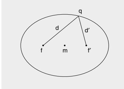
The characteristic property of the ellipse: The sum of the distance from an arbitrary point  $q$  on the perimeter, to the two foci  $f, f'$ , is a constant:
