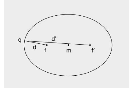
To determine the value of the sum of distances, consider the case, where  $q$  approaches the point on the major axis opposite  $f$ . At that point, we can see that the total length  $d + d'$  will be equal to the major axis of the ellipse:
