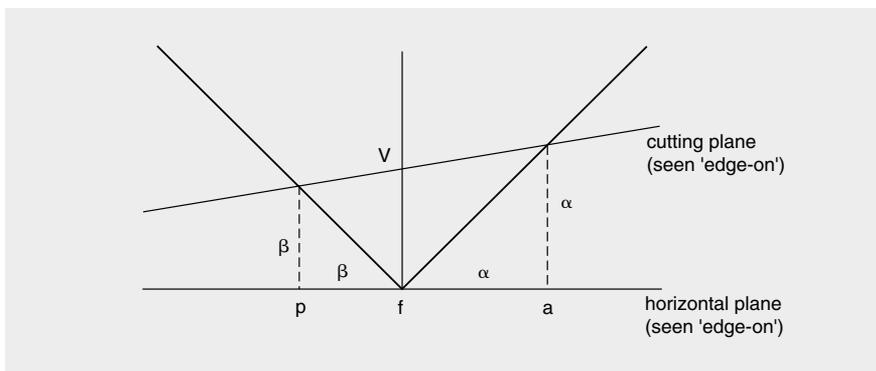
its height, which is equal to  $D$ , coincides with  $fV$ .) Those skillful in geometry can easily determine the length  $fV$  in terms of  $\alpha$  and  $\beta$  from the diagram.
