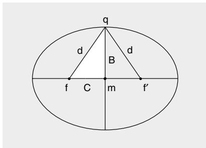
Applying the Pythagorean Theorem to the right triangle  $mfq$ , we find, that  $d^2 = B^2 + C^2$ . Since length  $d$  from focus  $f$  to  $q$  is equal to the semi-major axis  $A$ , and the total length  $d + d = 2A$ , we have the relationship between the semi-major axis  $A$ , the semi-minor axis  $B$ , and the
